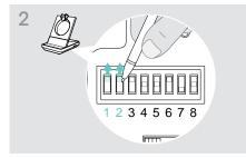
Use a pointed object to set the DIP switches 1 and 2 to the position shown.
