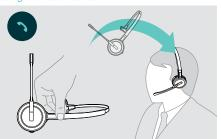
Lift the headset from the desk and put it on. The sensor registers motion and the incoming call is accepted.
