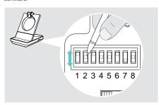
To configure the system via the DIP switches:
