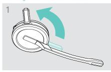
> Rotate the headset's charging pin away from the microphone boom.
