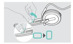
> Rotate the cheek spacer to increase or decrease the distance between the microphone and your mouth - if
