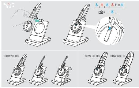
▶ Place the headset into the magnetic holder of the base station. The headset is paired to the base station, the LED flashes blue and red. The LED turns blue when pairing is complete and the headset will start charging.
