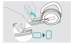
> Rotate the cheek spacer to increase or decrease the distance between the microphone and your mouth - if required.
