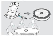
To use an external speaker with microphone such as the EPOS speakerphone SP 20:
