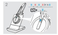
If the headset and base station are not paired, the headset LED flashes blue and red shortly. The LED turns blue when pairing is complete and the headset will start charging.
