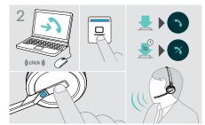
Press the hook button on the headset for 1 second. The voice prompt "Call rejected" is announced. The LED stops flashing and is fixed white.
