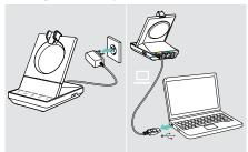
Disconnect the base station from the mains power supply and the computer.
