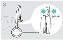
> Snap the charging pin into the headband.
