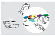
Connect the USB cable to the PC socket on the base station.
