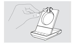
Delean the charging contacts of the base station and the headset from time to time using e.g. a cotton swab.
