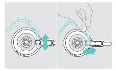
> Adjust the neckband's height and angle.
