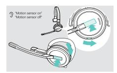
Press the volume button as shown and simultaneously the hook button. Hold the buttons until you hear three
