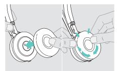
Attach the new ear pad to the ear cup by pressing firmly around the ear pad.
