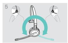
> Rotate the microphone boom to change wearing side.
