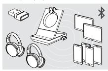
The dongle can save up to eight paired Bluetooth devices. If you pair a ninth device, the saved connection profile of the least used Bluetooth device will be overwritten. If you want to re-establish a connection with this device, you have to pair the devices again.
