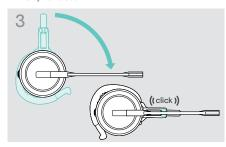
> Rotate the boomarm to snap it in the wearing style adapter.
