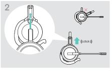
▶ Insert the charging pin into the holder of the wearing style adapter.
