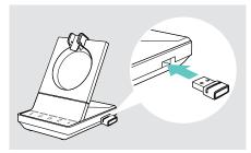
▷ Insert the BTD 800 USB into the USB port on the base station. Some older dongle versions need to be connected directly to the computer in order to be updated. "New" dongles can be identified by the two grey lines on the bottom side of the housing.
