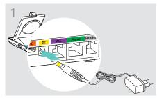
Connect the plug of the power supply unit to the DC socket (marked yellow).
