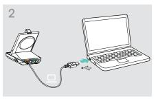
Connect the USB cable to a USB socket on your computer.
