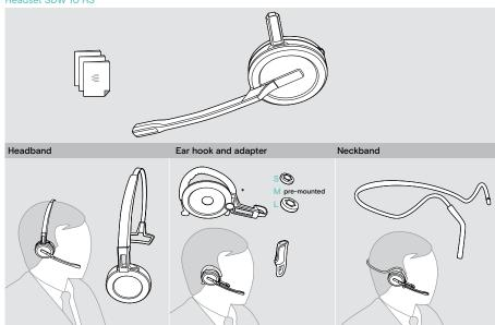
\*The wearing style adapter is also needed for assembling the neckband (see page 21).
