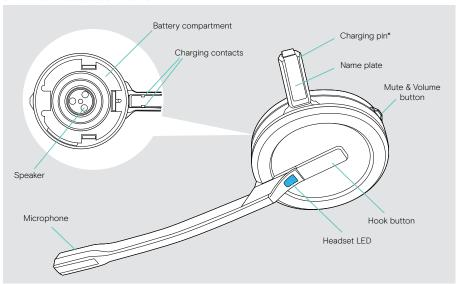
\*Inserted into the holder of the headband or wearing style adapter
