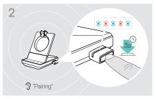
> Press and hold the dongle's button for 3 seconds to enter pairing mode. The LED alternately flashes blue and red.
