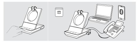
▶ Touch the icon of the desired audio source on your base station 每/□/□. The chosen audio source is in focus and the LED lights up white.
