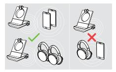
After switch-on, the dongle automatically tries to connect to the two last connected Bluetooth devices - mobile phone and headset cannot be combined. You can only connect a third Bluetooth device after having switched off the first or the second Bluetooth device.
