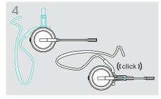
▶ Rotate the boomarm to snap it on the wearing style adapter like shown.
