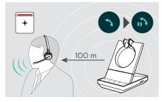
In office buildings, the range between DECT headset and base station is up to 100 m. Further information on how to adjust radio range is given on page 27.
