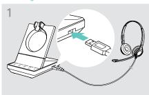
Connect the headset to the USB socket on the base
