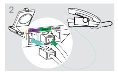
Connect the handset lifter to the ACC socket on the base station.
