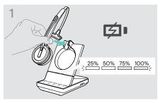
Place the headset into the magnetic holder of the base
