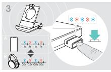
Press the button again to switch between pairing mode for mobile phones A or headsets B.
