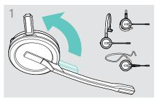
▶ Rotate the holder with the charging pin away from the microphone boom.
