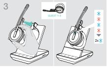
Press and hold the Mute & Volume button while placing the GUEST headset into the base station of the MASTER
