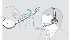
▶ Bend and rotate the microphone boom so that the microphone is about 0.8" (2 cm) from the corner of your
