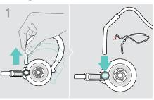
> Remove the ear hook from the wearing style adapter and insert the neckband instead. Make sure the inserted side has the holder mounted on the neckband.
