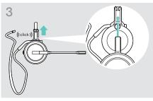
▶ Insert the charging pin into the holder of the wearing style adapter.
