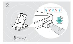
> Press and hold the dongle's button for 3 seconds to enter pairing mode. The LED alternately flashes blue and red.
