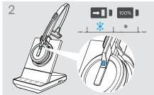
During charging the Headset LED lights up blue. The LED switches off when the headset is fully charged.
