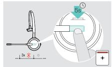
Press and hold the hook button for 5 seconds to switch off the headset. The Headset LED flashes red 3 times. The Headset battery status LEDs on the base station switch off. The + LED lights up red.
