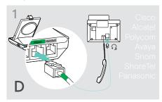
Connect the base station to the fixed line phone as shown in the cable Quick Guide.
