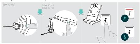
▷ Press the Mute & Volume button on the headset OR SDW 30 HS | SDW 60 HS: Mute button on the boom arm OR Touch the Mute button 4 on the base station.
