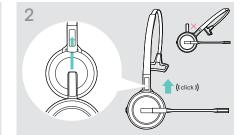
Slide the charging pin into the holder of the headband.
