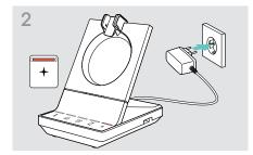
Connect the power supply unit to a wall socket. The + LED lights up red.
