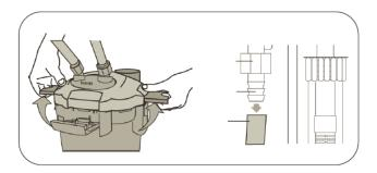
Remove the other hose at the tap. Now place one hand over the tap where the hose has been removed and blow into the hose.
