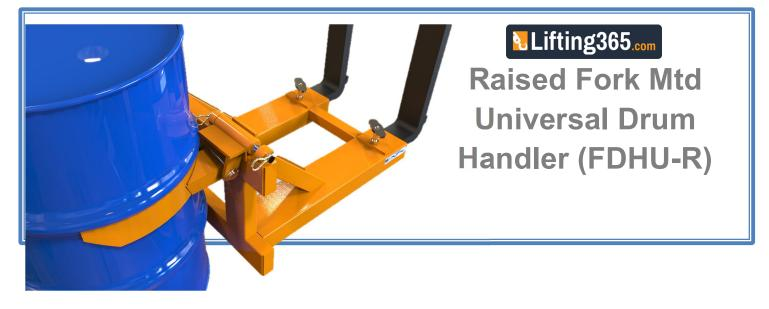
Fully automatic action, the attachment has two curved arms which hinge at one end. To lift a drum, approach it with the clamp arms horizontal and postioned halfway up the drum, between two rolling hoops. When the arms contact the drum they will open automatically, falling back around the drum as you proceed forwards. When the attachment is raised the arms will grip the drum tightly under the upper rolling hoop.
