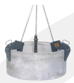
Torsionally rigid, light-weight hollow steel construction for the transportation and placement of manhole rings. The pipe tackle complies with official labour safety regulations and is equipped with a safety lock. Inadvertent slipping of the load through the claws is prevented by a spring on each clamp.
