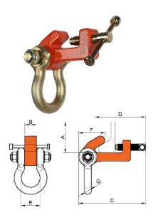
The Tiger BCB bulb bar anchor is designed for attaching to bulb profiles of bulb flat bars approved for lifting applications. These are often found in ship compartments, engine rooms and overhead bridge deck structures. The bulb bar anchor provides a semi-permanent lifting point. The large integrated shackle gives easy connection for all different types of lifting machines. This model must NOT be used for lifting beams. It is a suspension point.
