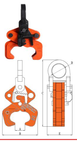
The Tiger CRT rail clamps are designed to lift single rails lengthways and crossways, securely and safely. The clamps are designed to fit most types of rail section currently in use. The clamps are locked onto the rail-head via a lever operated spring mechanism. Very solid, practical design with low dead weight. For rail sizes S49, S54, S60s, UIC60.
