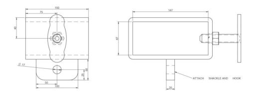
CONTACT Adjustable Fork Mounted Hooks are the most cost effective way of safely hanging a load under the forks of your lift truck. Simply clamps on the forks anywhere along there length.
