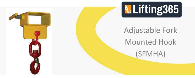
Single Fork adjustable hooks offer a low cost solutuion to your laod handling needs. The attachment fits quickly and easily to the fork truck to enable loads to be hung under the forks at any point along their length. Simply slide the attachment onto the forks and slide along until the desired load centre is achieved. Then simply screw the fork clamp tight. Ensure the attachment is secure before attaempting lifting.
