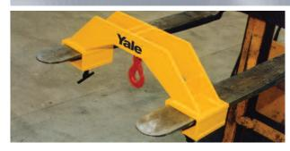
The FLTH tine hook is designed to convert your forklift truck into a crane. This is done by simply sliding the FLTH over the tines of your forklift truck and then fastening the tines by tightening the two threaded bars underneath. The unit is supplied as standard with a swivel safety hook.
