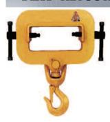
**The TZH tine hook** is designed to convert your forklift truck into a crane. This is done by simply sliding the TZH onto a single tine. The tine hook is fastened to the tine by tightening the two threaded bars on either side. The unit is supplied as standard with a swivel safety hook.
