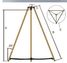
The Camlok Shearlegs have been designed to be simple, easy to erect and operate. Each set of shearlegs are supplied fitted with safety chains and a large eyebolt for the suspension of hand operated lifting devices
