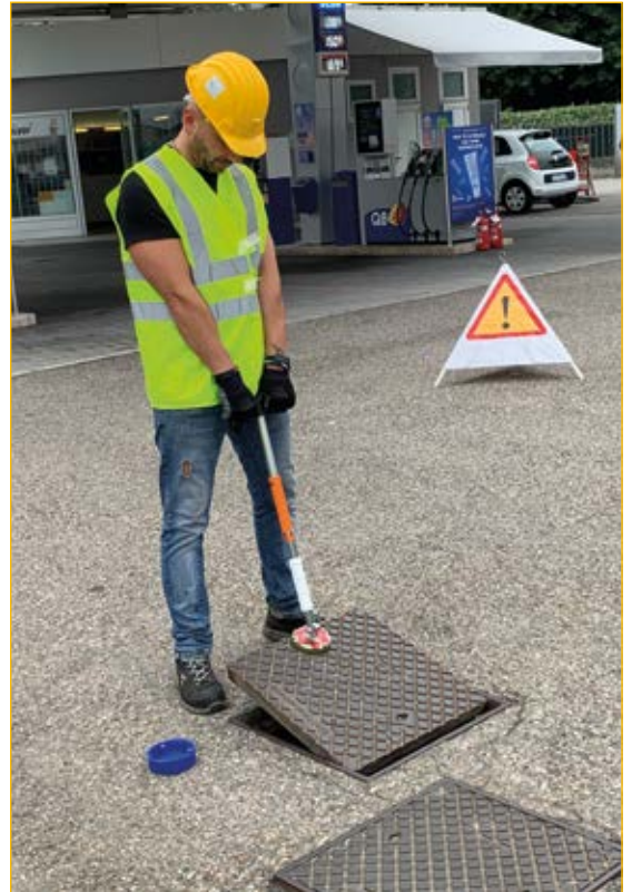
Category 3 ATEX tools suitable for use in places classified ZONE 2.
