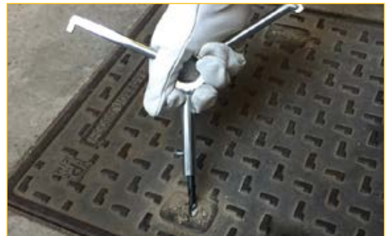
Configuration 1: with flat drill bit hook to clean and scrape.
