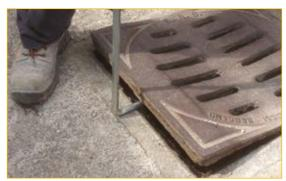
The "D" shapped handle provides a fulcrum point to facilitate the lifting operation.
