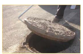
Built in tempered 38NCD4 steel with galvanized anti rust finish which makes the LB7 a resistant and robust tool.
