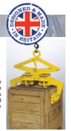
NB: When using the models fitted with rubber pads, it is important that the surfaces are dry, clean and free of oil and grease.
