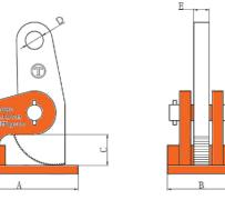
The Tiger CPH clamp is a horizontal lifting clamp intended to be used in pairs, sets of pairs, or in a tripod arrangement for transporting steel plates horizontally. They can be used to lift all types of materials in plate form providing that the plate can withstand the forces imposed on it. These clamps are only suitable for lifting single plates with a surface hardness below 300 Brinell (HB) / 32 Rockwell C (HRC).
