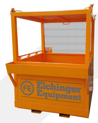
The 1074 4 Man Cage is built primarily with safety in mind, the cage conforms fully to BSEN 14502 and PM28. This cage has solid walled sides to half height and close mesh to the rear to prevent accidental injury but maintain visibility. The cage also benefits from internal overhead harness points.
