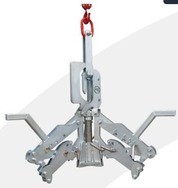
The 1067 manhole ring lifter has been designed to enable the safe movement of concrete ring products without the requirement of additional staff to couple or un-couple the unit during loading / unloading.
