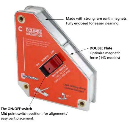
**NOTE:** Must be used for tack welding only and removed before completing weld. Avoid prolonged exposure of magnetic products to heat sources of 356°F / 180°
