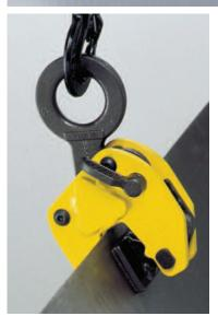
The LJ non-marking plate clamps are designed for lifting, turning and transporting of structural steel plates, stainless steel, iron, timber and aluminium without marking, damaging or leaving indentations on the surface. It can also be used for steel plates with extremely hard surfaces.
