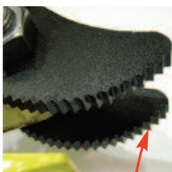
CH with serrated jaw which can only be used for single plates, NOT bundles
