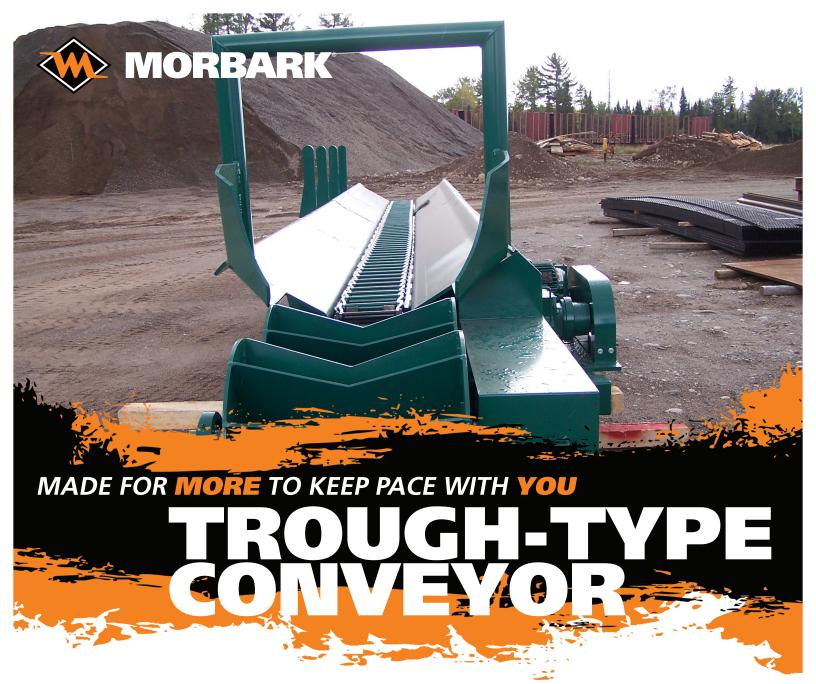
These heavy-duty log conveyors are used in a variety of applications, including sawmills, chip plants and log merchandizing systems. Morbark offers **Trough-type Conveyors** built from 0.5" (a.3 cm) or 0.62" (1.6 cm) formed steel plate in a variety of lengths and widths. Several different drives are available, as well as automatic or manual kickers.
