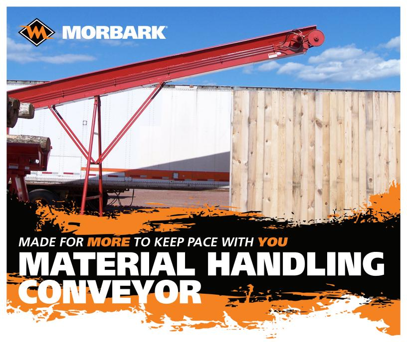
This heavy-duty, versatile, paddle-type conveyor is available in widths of 14" (35.6 cm) and 24" (61 cm) and lengths up to 100' (30.5 m). The conveyor is fabricated from 10 gauge formed steel panning with enclosed chain return, with steel reinforced hardwood paddles on 24" (61 cm) centers.
