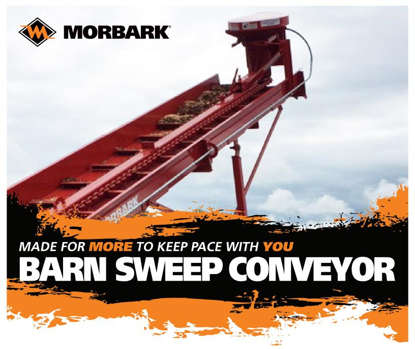
Perfect for transferring sawdust, bark or chips from one place to another, the **Barn Sweep Conveyor** is ideal when coupled with our Rosserhead Debarker. Constructed from 10-gauge formed steel pan and 5" x 5" (12.7 cm x 12.7 cm) square tubing, the barn sweep conveyor can be made up to 150' (45.7 m) level or 100' (30.5 m) upright.
