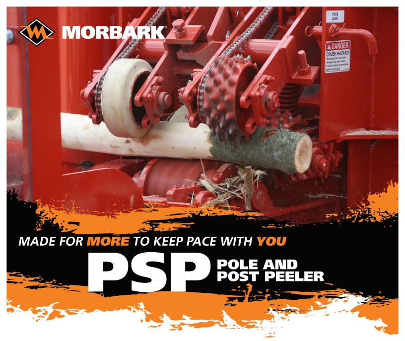
The **Morbark PSP Pole and Post Peeler** peels logs from 6' to 25' in length (1.8 m – 7.6 m) and 3" to 12" in diameter (7.6 cm – 30.5 cm). It can peel up to 40 feet per minute (12.2 m/min). All Morbark post peelers use a split peeling head with carbide-tipped cutterhead teeth to remove bark and knots and planer knives to provide a smooth surface with only one pass through the machine.
