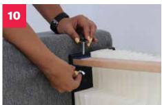
Rotate the thumb screw with the wing nut together.
