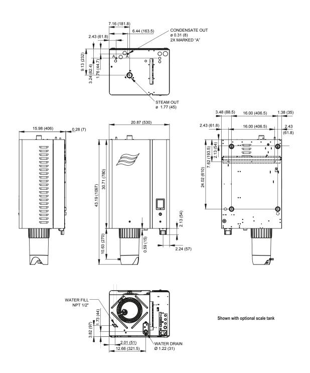
Fig. 22: Unit dimensions unit "Medium"- dimensions in Inch (mm)
