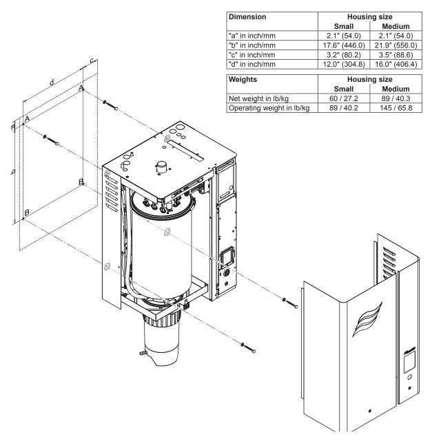
Fig. 7: Overview standard mounting single units Small and Medium
