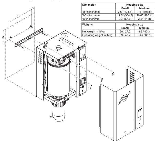
Fig. 9: Overview wall support mounting single units Small and Medium
