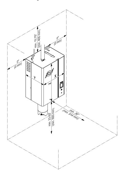
Fig. 6: Minimal clearances to be observed
