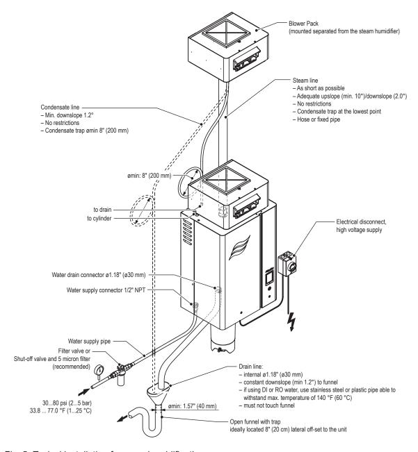
Fig. 5: Typical installation for room humidification
