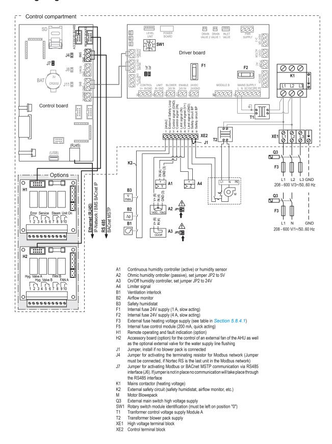
Fig. 19: Wiring diagram Nortec RS - Single units Small and Medium
