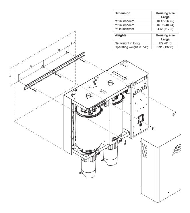
Fig. 10: Overview wall support mounting single units Large
