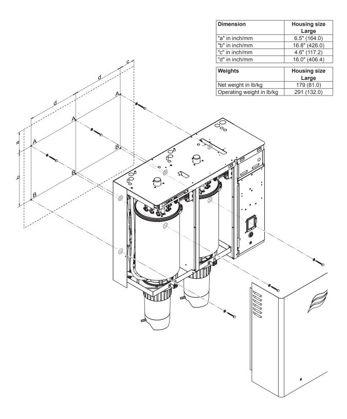
Fig. 8: Overview standard mounting single units Large
