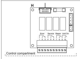
The remote operating and fault indication board contains four potential-free relay contacts for the connection of the following operating and fault indications:
