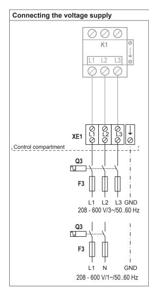
The voltage supply (L1, L2, L3 and GND or L1 and) is to be connected in accordance with the wiring diagram to the corresponding terminals of the main contactor in the control compartment. The earth conductor is to be connected to the earth terminal right beside the main contactor. The supply wiring is to be fed into the unit via the clamp strap on the bottom of the unit. Note: Double units have separate heating voltage supplies for each steam cylinder.
