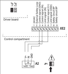
The signal cable of an ohmic humidity controller  $(140\Omega...10k\Omega)$  is to be connected according to the wiring diagram to the terminals "3" (GND), "4" (IN) and "6" (V+) of the control terminal block "XE2" inside the control compartment.
