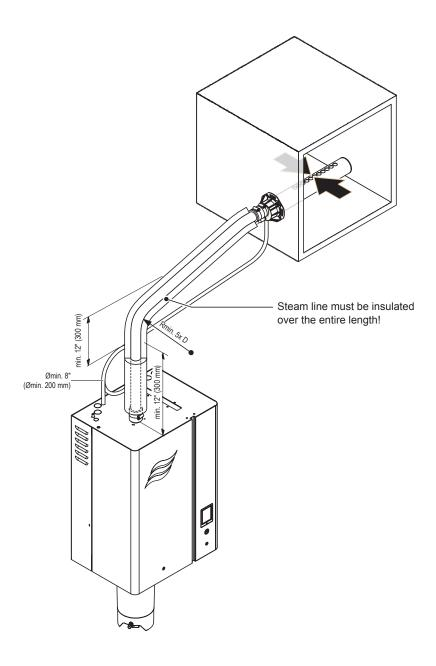
Fig. 15: Steam line with solid piping and insulation
