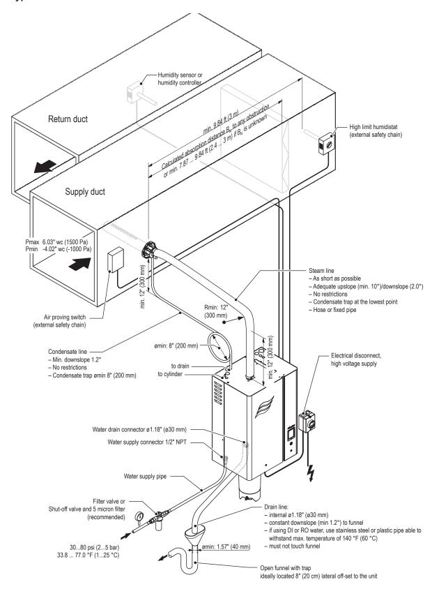
Fig. 4: Typical installation for duct humidification
