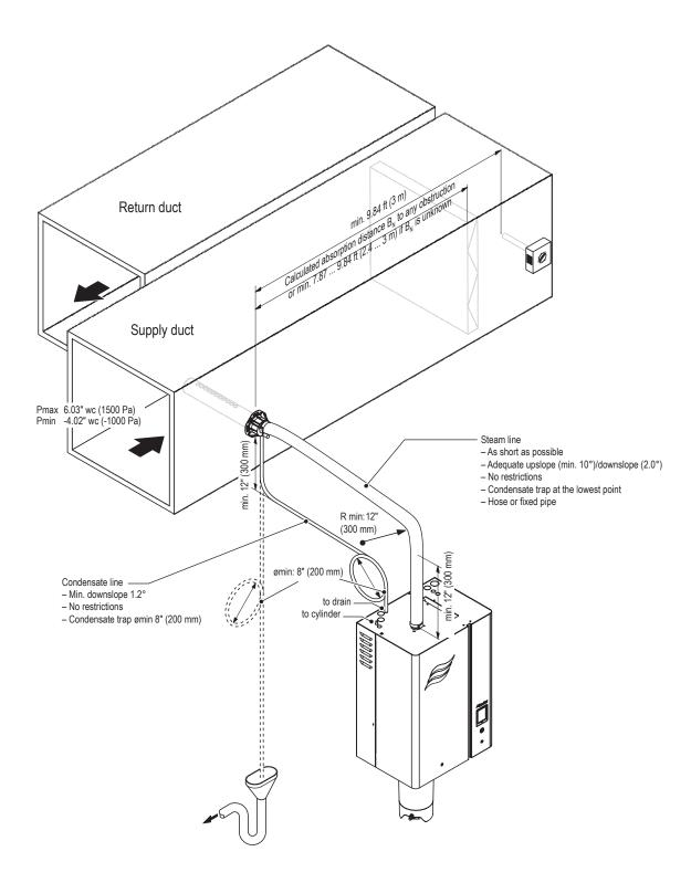
Fig. 11: Overview steam installation for duct humidification
