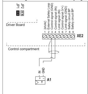
The signal cable of an external controller or of a humidity sensor (if the internal P/PI controller is used) are to be connected according to the wiring diagram to the terminals "3" (GND) and "4" (IN) of the control terminal block "XE2" inside the control compartment. The admissible signal values can be found in the technical data table in the operation manual. The connecting cable must be led through a cable gland into the control compartment.
