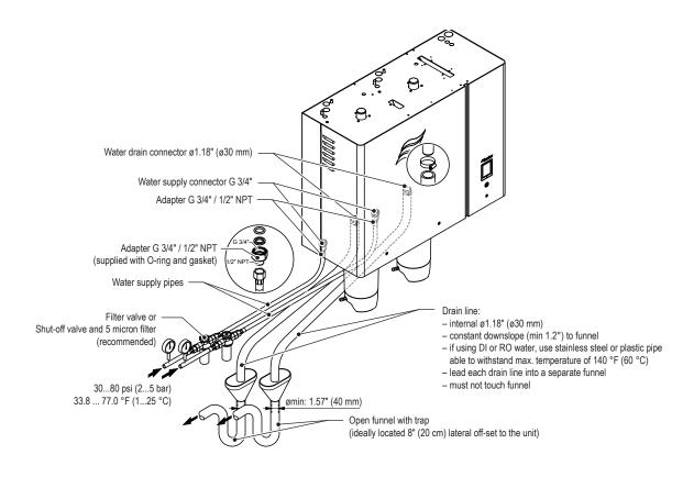
Fig. 17: Overview water installation for single units Large
