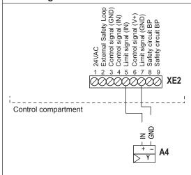
The signal cable of an external limiter (P/PI continuous controller) is to be connected according to the wiring diagram to the terminals "5" (Limit signal IN) and "7" (Limit signal GND) of the control terminal block "XE2" inside the control compartment.
