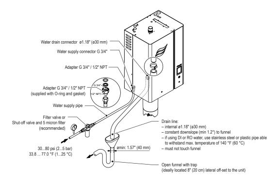
Fig. 16: Overview water installation for single units Small and Medium
