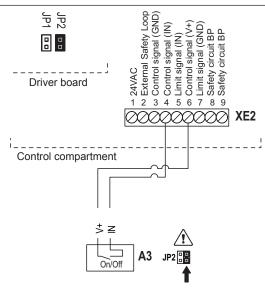
The signal cable of 24V On/Off humidistat is to be connected according to the wiring diagram to the terminals "4" (IN) and "6" (V+) of the control terminal block "XE2" inside the control compartment.
