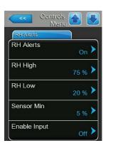
**RH Alerts**: with this setting you can activate ("On") or deactivate ("Off") the output of a warning upon malfunction of the humidity sensor.
