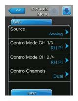
Source: with this setting you determine the source of the control signal.
