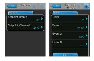
Activate the timer function (Setpoint Timers: **"On**"). If the setpoint timer is activated, up to eight switching points (Event 1... Event 8) with different humidity setpoints can be defined. Each switching point is defined by a weekday or weekday range, the switching time and the humidity setpoint in %rh.
