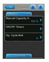
Manual Capacity A: with this button you can access the settings menu for the capacity limitation. Here you determine whether the Nortec RS is to be operated with a fix capacity limitation (factory setting) or whether it is to be operated with a timer controlled capacity limitation.
