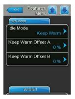
Idle Mode: with this setting you determine the operational behaviour of the Nortec RS in standby operation.
