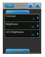
**Contrast**: with this setting you determine the desired value for the display contrast.
