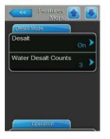
Desalt: with this setting you can activate ("On") or deactivate ("Off") the demineralization mode.
