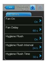
**Fan On**: with this setting you can activate ("On") or deactivate ("Off") the control of an external fan via the corresponding relay on the optional accessory board.
