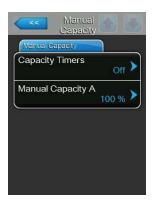
Let the timer function deactivated (Capacity Timers: "Off") or deactivate the timer function if necessary. Then, set the desired capacity limitation of the steam humidifier in % of the maximum capacity via the "Manual Capacity A" parameter (Factory setting: **100** %, Setting range: **20** ... **100** %).
