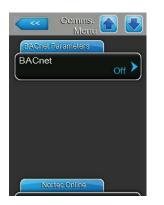
**BACnet**: with this setting you can activate ("MSTP" or "BACnet/IP") or deactivate ("Off") the communication via the integrated BACnet interface. Note: in order to activate the setting of this parameter the Nortec RS must be switched off and on again.
