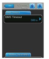
**BMS Timeout**: with this setting you determine the maximum time the humidifier will wait with no communication from the BMS network before a BMS timeout warning is generated. Exceeding the timeout also stops humidifier operation if the signal source of the humidifier is set to a BMS input.
