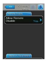
Allow Remote Disable: with this setting you can activate ("Yes") or deactivate ("No") remote blocking via the BMS.
