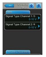
**Signal Type Channel 1/3**: with this setting you determine the control signal with which the steam humidifier is controlled.
