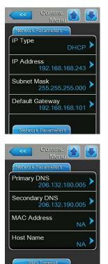
The following network settings are used only for the communication via the integrated BACnet IP interface.
