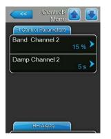
**Band Channel 2**: with this setting you set the proportional range for the internal P/PI supply air controller in %rh. **Note**: this setting appears only if the "Control Mode" is set to "RH P" or "RH PI" and "Control Channels" is set to "Dual". Factory setting: **15**%
