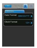
Date Format: With this setting you determine the desired date format. Factory setting: DD/MM/YYYY
