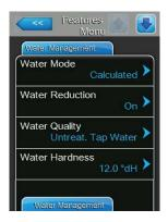
The following settings appear only, if **"Water Mode"** is set to **"Calculated"**. **Important:** the water quality and the water hardness of the supply water must be known. Using wrong values for these two parameters may lead to increased maintenance work and operating malfunctions.
