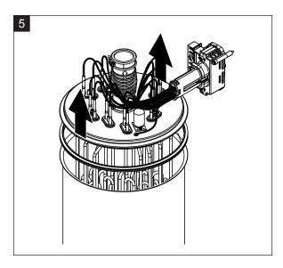
5. Carefully lift off the cover with the heating elements.
