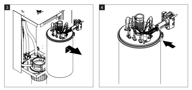
3. Carefully lift the steam cylinder out of steam cylinder receptacle and remove it towards the front of the unit.
