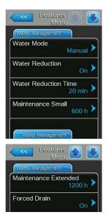
The following settings appear only, if **"Water Mode"** is set to **"Manual"**. Note: The settings for the parameters to be selected depend on the supply water quality and the steam capacity of the unit and must be set in accordance with the following table. It may have to be adapted to the actual circumstances during operation.
