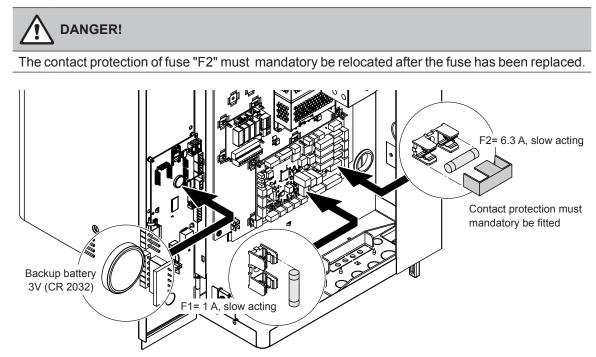
Fig. 6: Position of the backup battery and the fuses on the driver board
