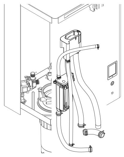
1. Release hose clamps, then disconnect all hoses from the corresponding connectors and remove the hoses.
