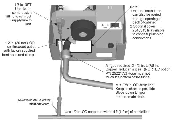
\*Pipe and water shut-off valve not supplied by Nortec.
