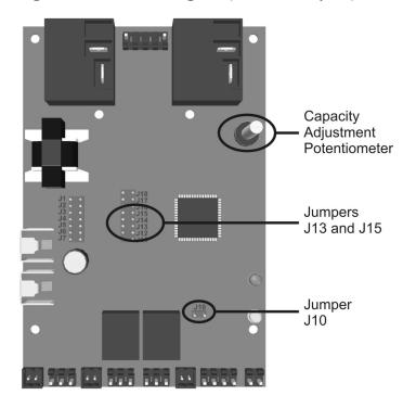
Figure 31: RH2 Control Board Jumpers
