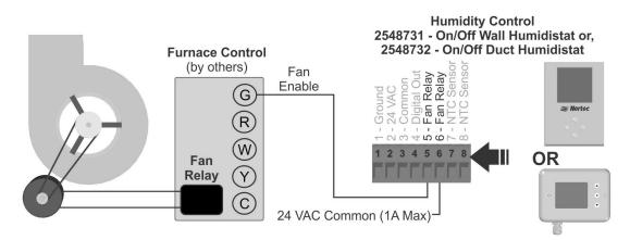
Figure 23: Digital On/Off Humidistat Fan Enable
