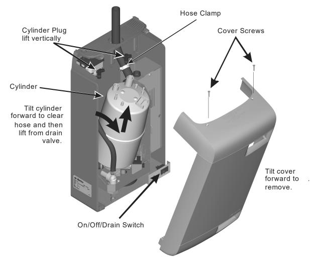
Figure 34: Cylinder Removal
