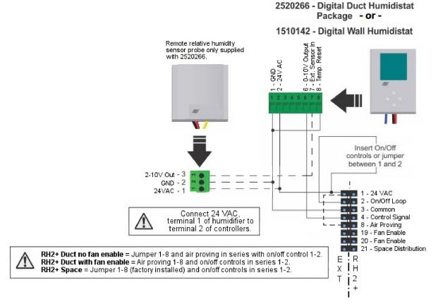
Figure 21: Modulating Control Wiring
