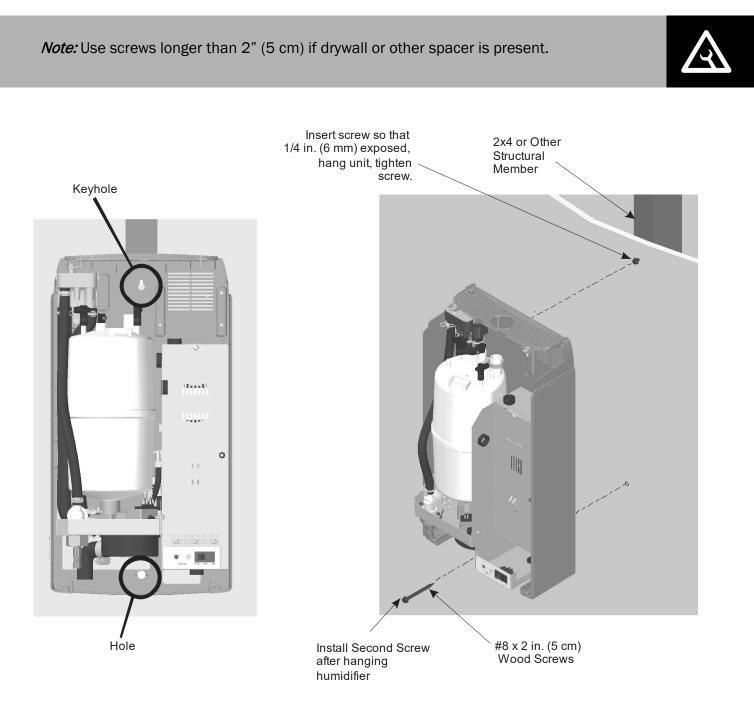
**Figure 5: Mounting With Keyholes**
