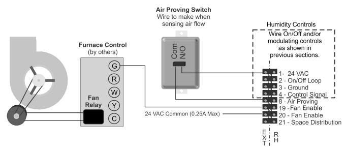
Figure 22: RH2+ Fan Enable Wiring
