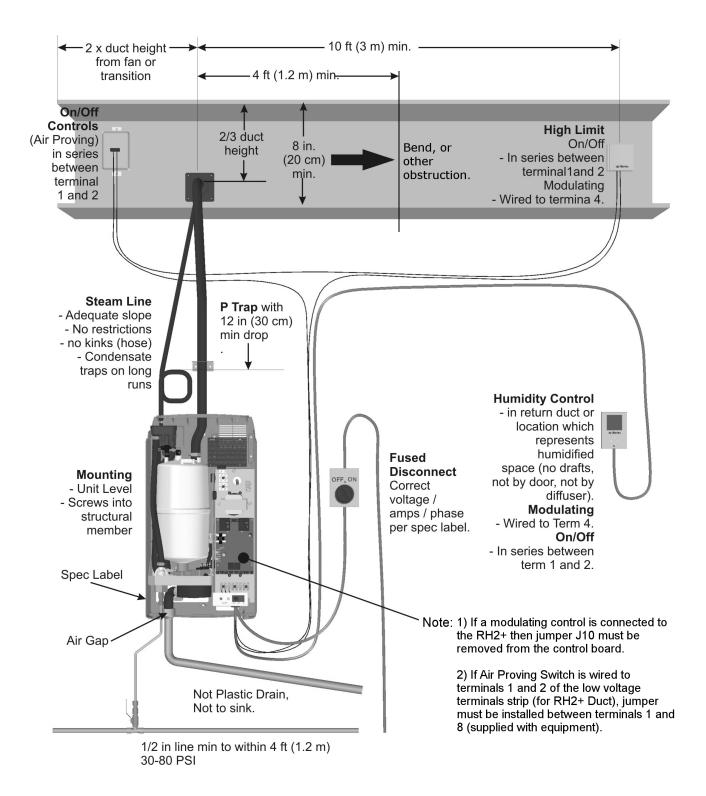
**Figure 25: Installation Check**
