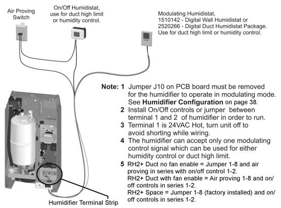
**Figure 20: Modulating Controls**
