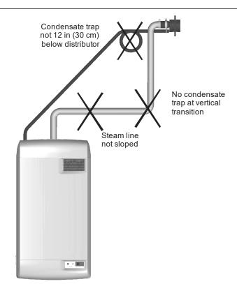
Figure 14: Common Steam Line Errors
