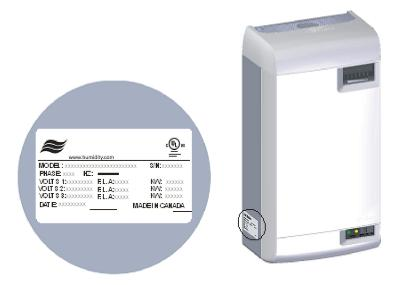
Figure 1: Specification Label Location
