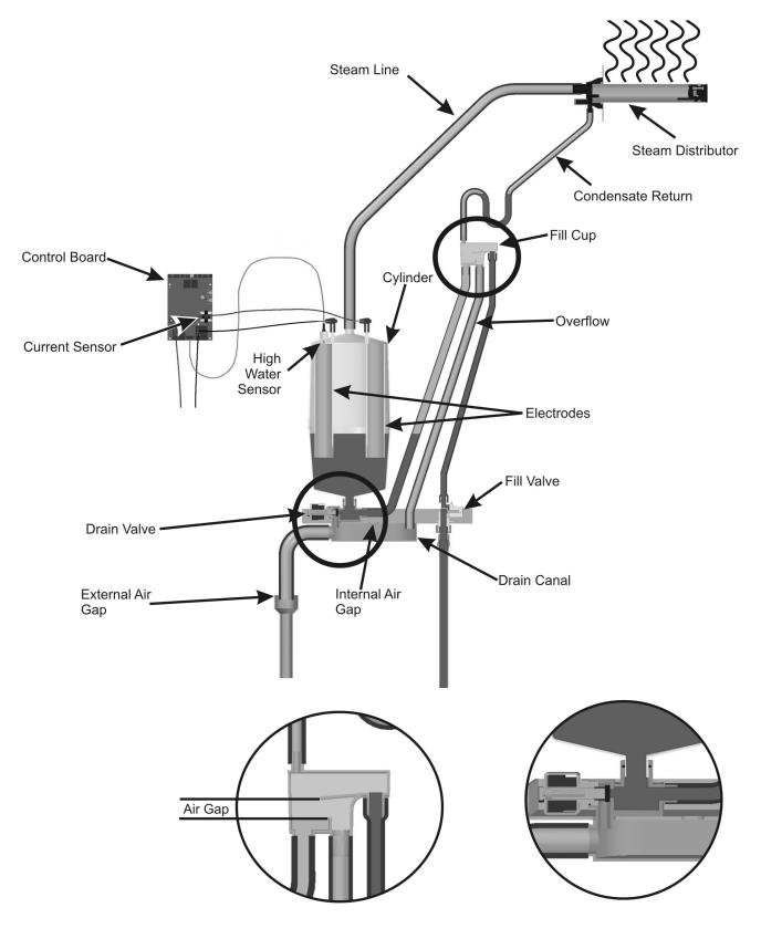
Figure 29: Humidifier Schematic
