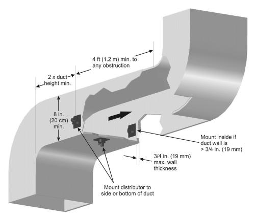
Figure 7: RH2+ Duct Nozzle Distributor Installation
