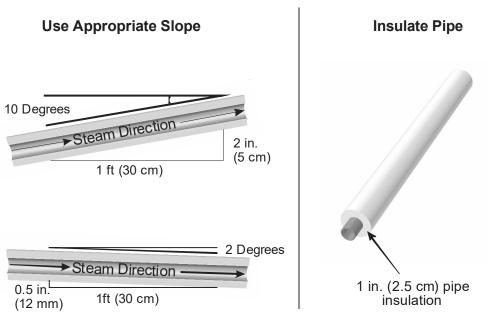
Figure 10: Main Steam Line Requirements
