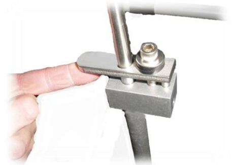
Slowly lift up lever on clamp block.
