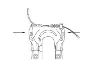
The brake blocks should be replaced if the oblique notches have worn away (further than the safety line (A)). If the blocks are in need of replacement, consult a bicycle specialist to get the correct type of brake blocks.
