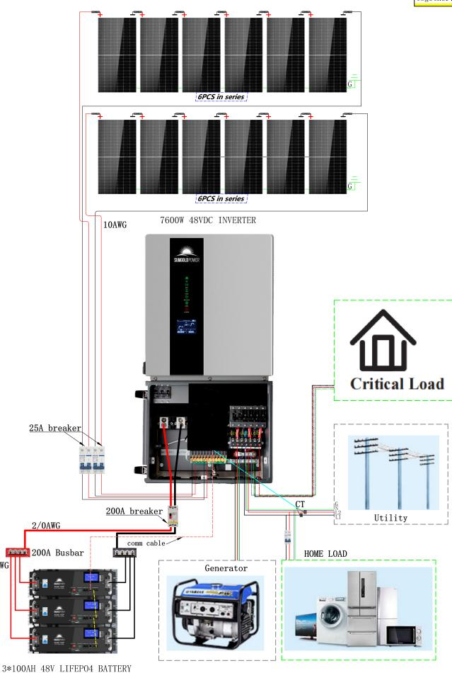
HYBRID SOLAR KIT 7.6KW 48V SPLIT PHASE 15.36KWH LITHIUM BATTERY 12 X 500 WATT SOLAR PANEL
