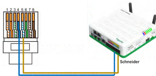
Connect with Schneider inverter/charger
