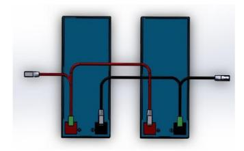
In parallel, it is recommended to use welding to connect.
