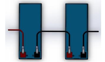
When battery is fixed in series, it is recommended to use the plug-in method for the connection. If the vibration is relatively large during use, it is recommended to use welding to connect.
