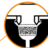
Filling Chamber properly filled
