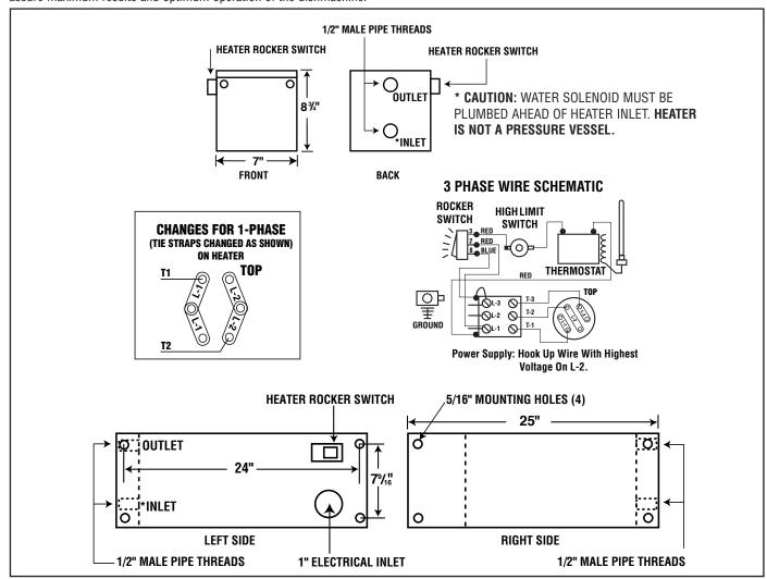
The CMA-Temp-SureTM option assures a continuous supply of 140°F hot water resulting in excellent dishmachine performance. The heater is custom-designed for fill and dump CMA single tank dishwashers as a factory added option or an infield add-on. The heater will also fit most competitor's single tank dishmachines
