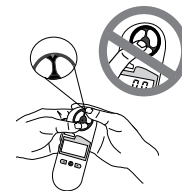
Replacing the Impeller
