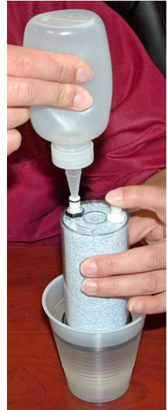
Figure 13: Checking Desiccant Cartridge for leaks.
