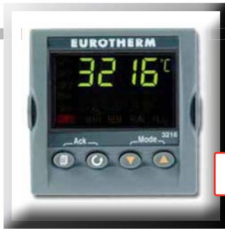
PID Control display system
