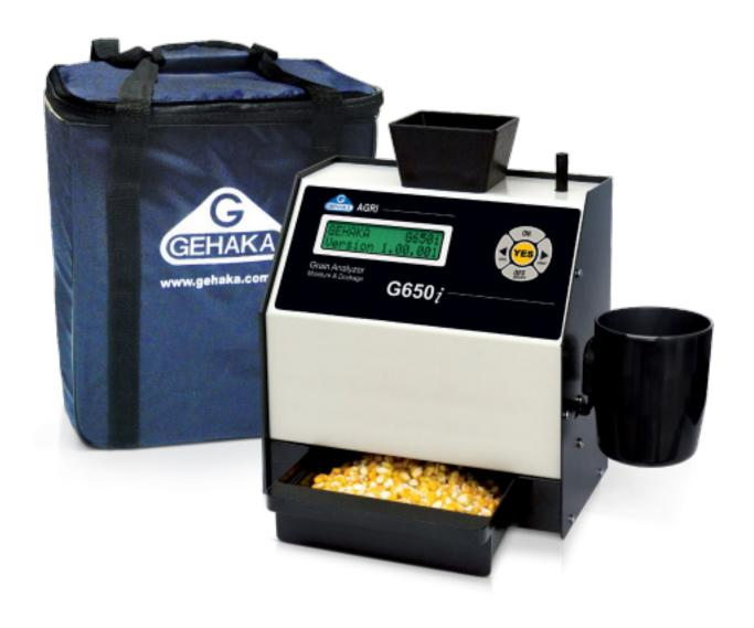
G650i Portable grain moisture, foreign material and test weight analyzer
