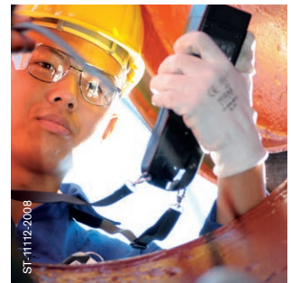
Dräger X-am® 5000 Optional external pump for clearance measurements.
