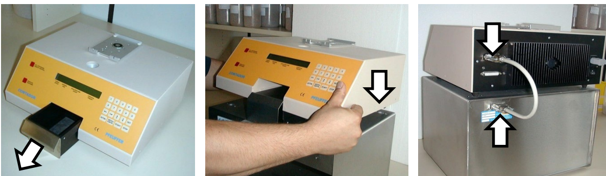
Figure 9: Put on CONTADOR and connect with CONTAFILL
