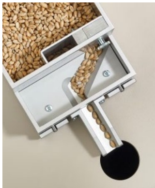
Figure 22: Flow of the seeds into the channel Start the count and observe the flow of the seeds.
