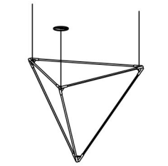
3 MOUNTING POINTS DIRECT-MOUNT TO CEILING (D3)
