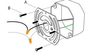
3] Make the wire connections from junction box wires to the Fixture while carefully holding the fixture. Push the connected wires back through the center hole of the Mounting Plate (A).
