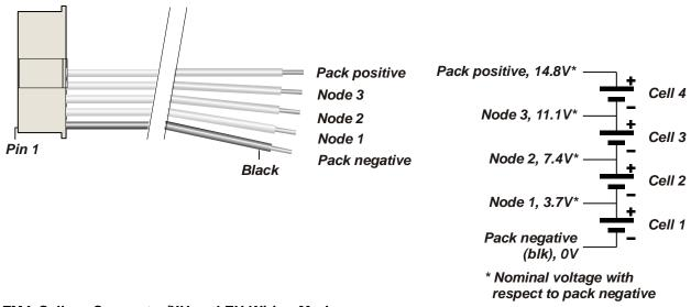
FMA Cellpro Connector/XH and EH Wiring Mode
