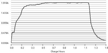
With the 1.0C Auto Current Mode, a fully discharged pack is charged to its nominal capacity in about 60 to 80 minutes, depending on the state of imbalance. Auto Current Mode takes into account a pack's starting charge level, so topping off a 50% discharged pack takes only about 30 minutes.
