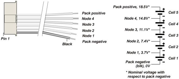
FMA Cellpro Connector/XH and EH Wiring Mode
