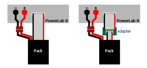
For non-balanced charging, connect the pack to Dual PowerLab 8x2 like this:
