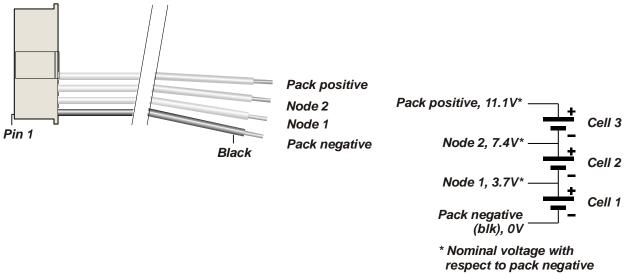
FMA Cellpro Connector/XH and EH Wiring Mode
