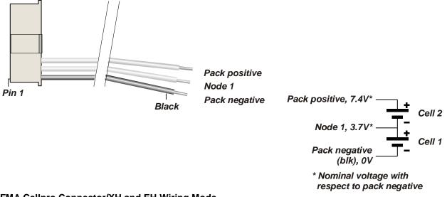
FMA Cellpro Connector/XH and EH Wiring Mode
