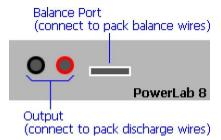
The Balance Port accepts a 9-pin Cellpro balance connector, which supports packs up to 8s. For charge/discharge rates up to 3A, you can attach just the balance connector, as shown below. If the pack has a different style balance connector, REVOLECTRIX offers a variety of adapters for most popular connector types and brands (visit the <u>Cellpro Adapters</u> section in the REVOLECTRIX Web site).
