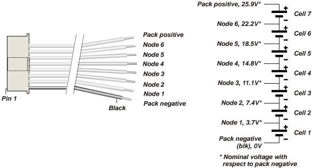
FMA Cellpro Connector/XH and EH Wiring Mode
