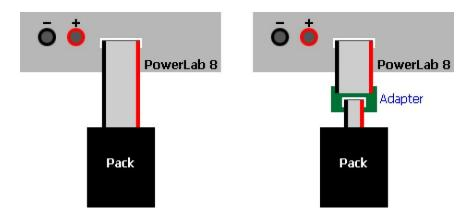
If the pack has both heavy discharge wires and a balance connector, you can connect both to Dual PowerLab 8x2 (good for any charge/discharge current):
