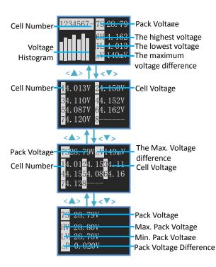
As the left pictures: the '7' in "7S" means cell counts; '6H' means the 6<sup>th</sup> cell voltage is the highest; '1L' means the 1<sup>st</sup> cell voltage is the lowest.
