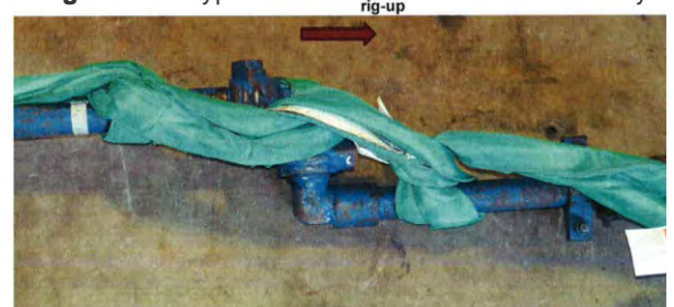
Figure 9. Typical Hitch on Swivel Assembly
