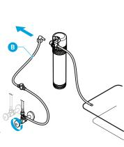
B. Connect the tip of the shut-off value tube (B) to the left side of the filter housing (C).
