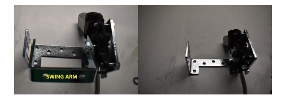
2.) Use 10mm wrench to remove (4) motor mount bolts. Rotate motor up 90 degrees and reinstall bolts to secure motor in vertical position as shown. If you have some, apply a little fresh blue loctite to the bolts during reassembly.
