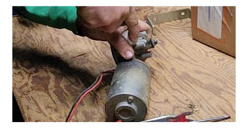
4.) Remove plate from the back of the gear box using a ¼" Nut Driver.
