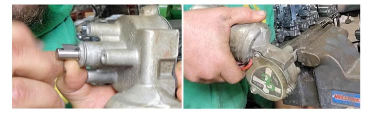
9.) Install motor back onto The Green Guard Base. Install the (3) ¼"-28 fine thread bolts and tighten using a 7/16" wrench. If necessary, install more blue Loctite.
