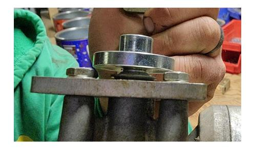
11.) Install blue Loctite in (4) threaded holes in coupling. Install Swing Arm. Install (4) little black 6-32 Allen head screws and tighten using 7/64" hex key wrench.
