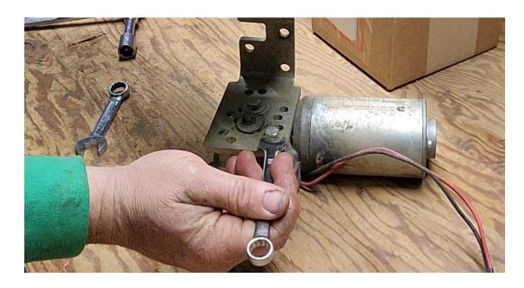
3.) Pry Spring Washer off of Motor using a flat blade screwdriver (This is what holds the shaft in place).
