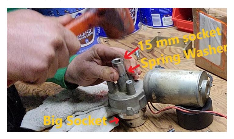
8.) Install new gasket and reinstall plate on back side of gear box.
