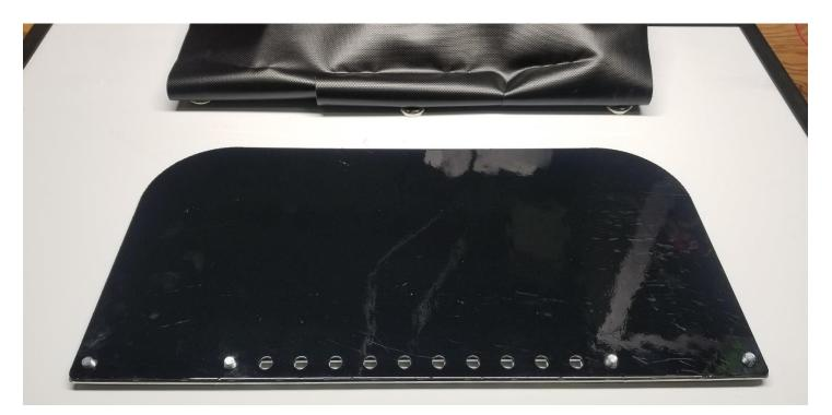
2.) Lay the Dust Blocker over the guard (with the magnet side down), and line the holes up. Install the supplied washers and reinstall the lock nuts. Tighten with a ½" wrench.
