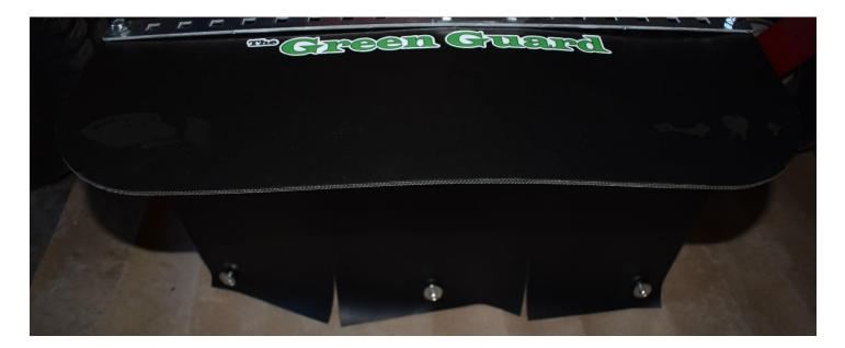
4.) Pull the magnetic end of the dust blocker up over the mower chute opening and stick the magnets to the top of the mower deck. Line up the slits in the dust blocker with the uprights on the green guard base, and secure the middle magnet to the green guard base. If you can't line up the existing slits, you can cut additional slits with a scissors.
