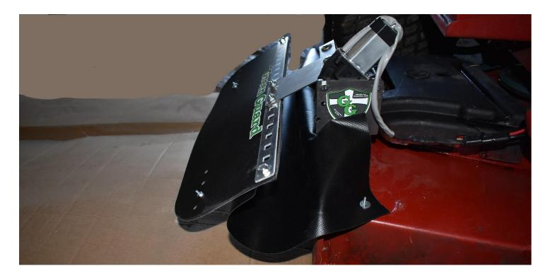
5.) Pull the magnets back from the edge as much as you can. Allow enough slack that the guard can open all the way, but tight enough that the excess material (when the guard is closed) won't enter the mower chute.
