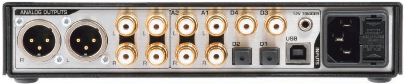
Photo 3: This is the rear panel of the DAC3 HGC. The digital inputs shown on the right include two S/PDIF coaxial, two TOSLINK optical, and one USB 2.0. Analog I/O includes two stereo RCA inputs, two stereo RCA outputs, and stereo balanced outputs. (Photo courtesy of Benchmark Media Systems, Inc.)
