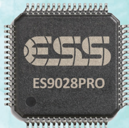
Photo 1: The 64-pin ES9028PRO digital-to-analog converter (DAC) chip is a drop-in replacement for the older ES9018. Total harmonic distortion (THD) compensation is among the significant improvements in the new chip. (Photo courtesy of ESS Technology)
