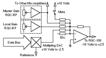
Figure 3. Possible Control Mix Amplifier Using RGC-RP
