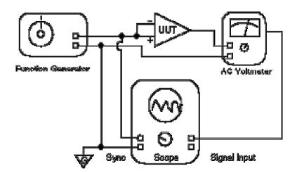
Figure 4. CMR Null Test Set-Up
