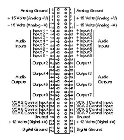
Figure 2. Rear View of RGC-108 Card Edge Connector Assignments
