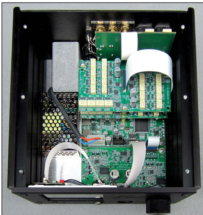
Photo 4: This is an inside view of the HPA4. The stacked left and right line amplifier circuit boards are visible toward the rear panel. Each line amp board contains active circuitry based on LME49860 op-amps and volume switching using gold-contact relays and 0.1% precision resistors. The THX-888 headphone amplifier board is on the bottom, toward the front. The digital control board is partially hidden by the analog boards, and the switching-mode power supply module is on the left.
