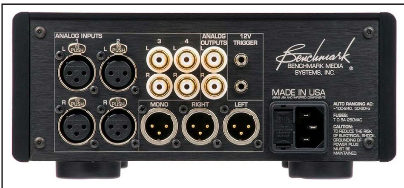
Photo 2: The rear panel of the HPA4 includes two stereo balanced XLR inputs and two stereo unbalanced RCA inputs. The fully-balanced outputs include stereo and summed-mono XLR connections, along with stereo unbalanced RCA connectors. The 12 V trigger connections can be used as either inputs or outputs, and the power connector accepts standard IEC power cords.
