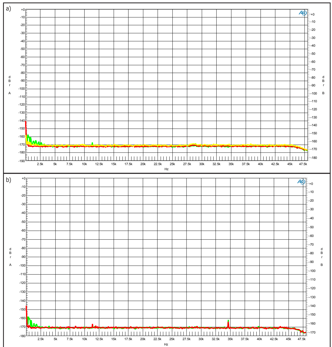
Figure 1: These graphs show FFT plots of the HPA4's idle channel noise, balanced in to balanced out (a) and balanced in to headphone out (b). Green is the left channel, red is the right channel, and yellow is the summed mono output in the top graph (a) only. The left and right scales are calibrated relative to +28 and +22 dBu, respectively. The graphs show that the headphone amplifier retains the exceptional noise performance of the line amplifier, with idle noise at or below -160 dB over most of the audible spectrum. All of Benchmark's measurement graphs are done with the Audio Precision AP2722. (Image courtesy of Benchmark Media Systems)
